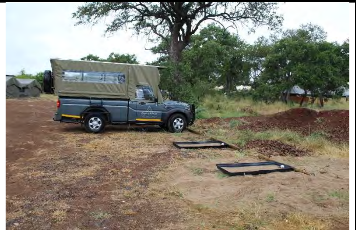
Figure 12: Vehicles: Parked over drip trays. Good.
