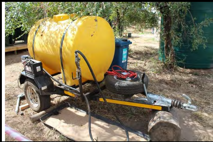
Figure 7: Generator Refuelling Bowser: Parked over a drip tray.
