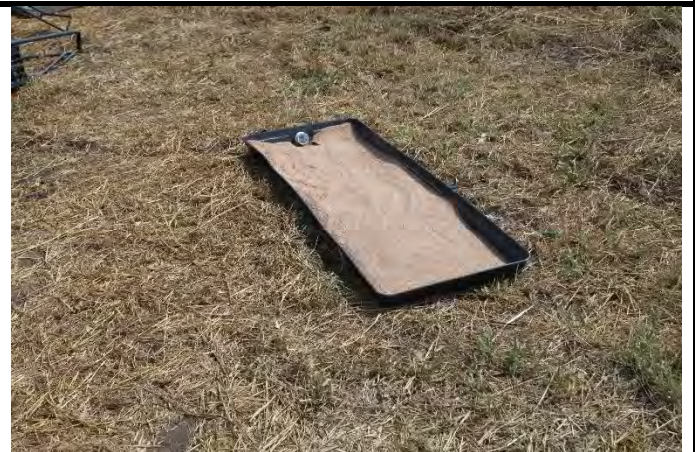
Figure 24: Drip Trays: Used at all applicable locations.
