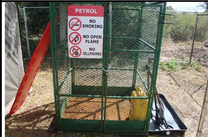
Figure 23: Hazardous Liquids Store: Locked and separate from other waste materials.
