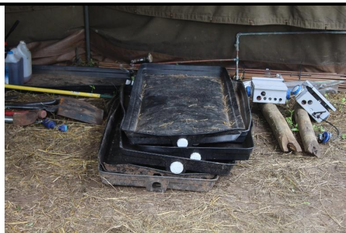
Figure 4: Drip Trays: On site and ready for use where applicable.
