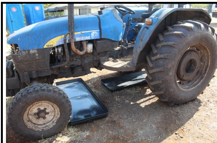
Figure 13: Drip Trays: On site and being used.
